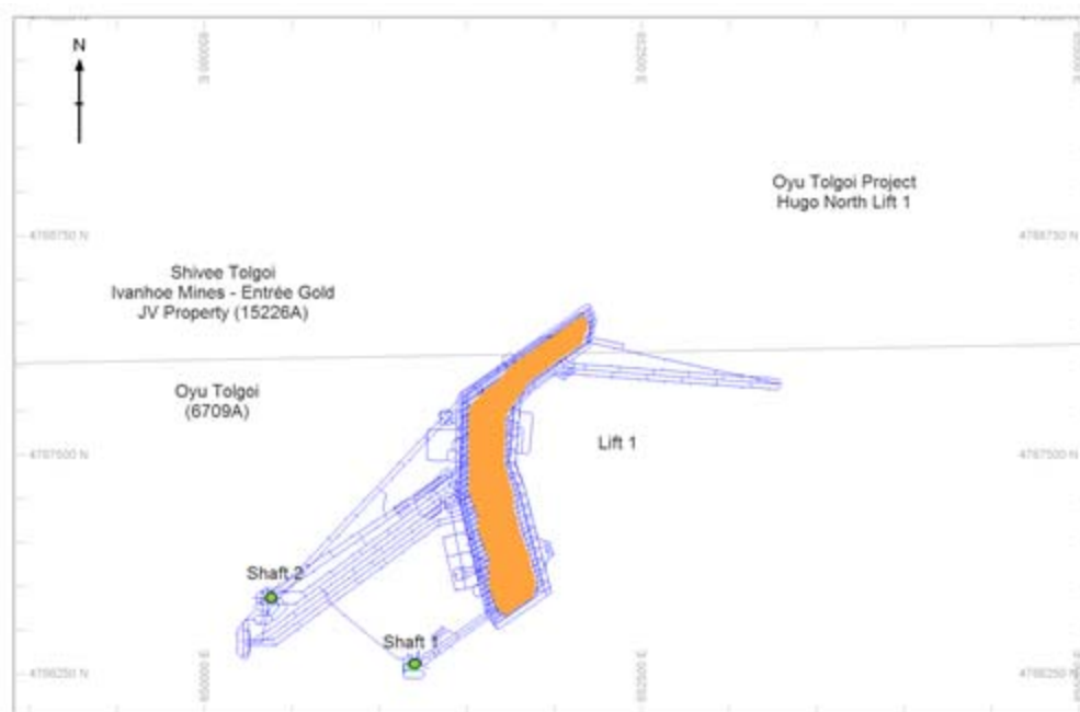
Figure 4 – Hugo North Lift 1 Block Cave Plan
